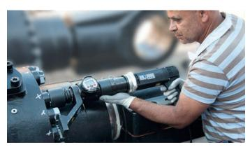
Optional accessories: The mobile measuring unit Torque Control
