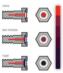
The indication is based on the deflection of an internal pin when the fastener is tensioned.
